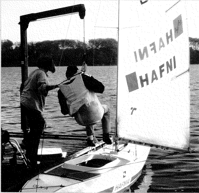
Using mechanical lift to get from dock to boat
